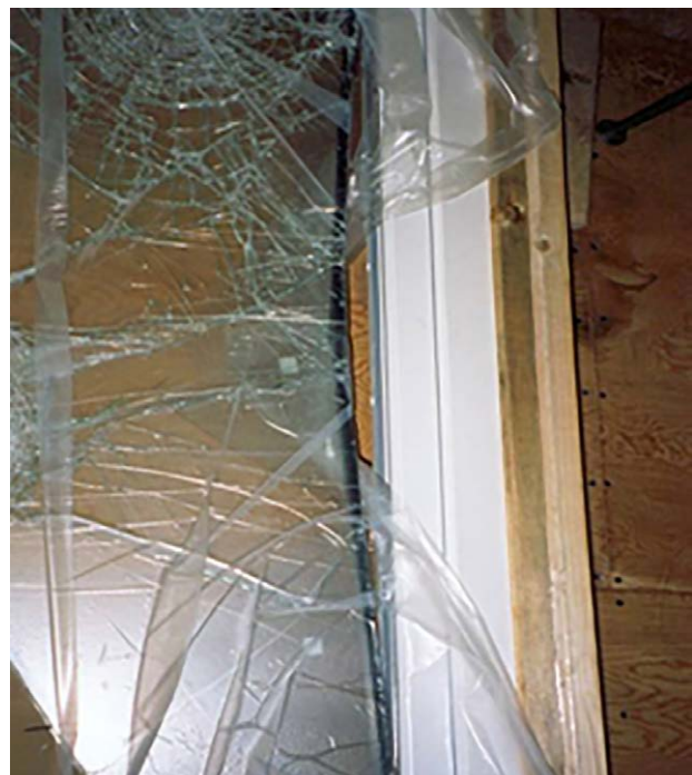
Fig. 13 Testing of hurricane-compatible components at ift Rosenheim according to [20] (Source: ift Rosenheim)
