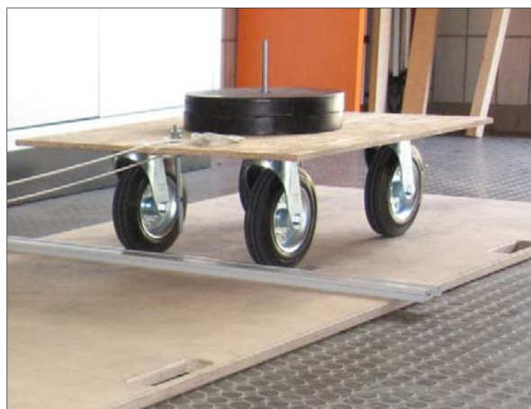
Figure 4 Realised trolley for testing the capability of rolling over thresholds. Additional weight 40 kg fastened in the middle of the panel. Position on the moving surface in front of the installed threshold.
