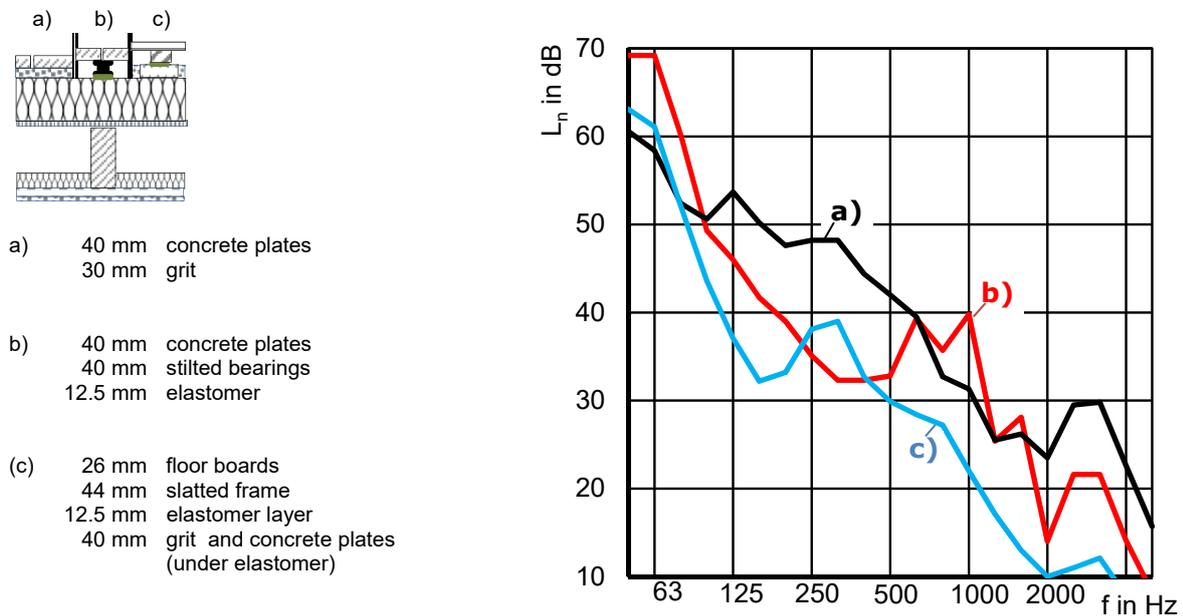
**Figure 6** Standard impact sound level of different constructions on a rafter / beam element with suspended ceiling and 140 mm EPS on-roof insulation panels
