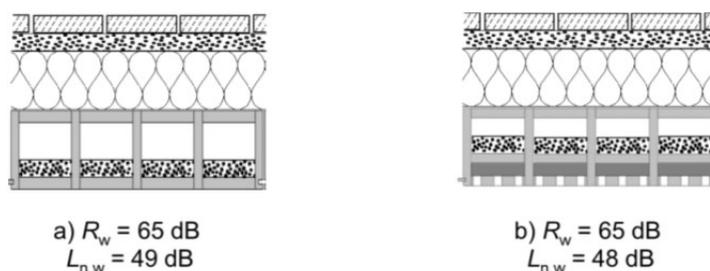
**Figure 2** Flat roofs made of solid wood box elements, EPS on-roof insulation, roof sealing and concrete plates in the gravel bed:
