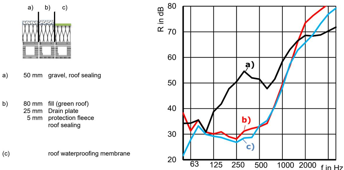
**Figure 4** Comparison of the constructions: Gravel roof, green roof and simple waterproofing membrane on a cross laminated timber - box element with 200 mm EPS on-roof insulation
