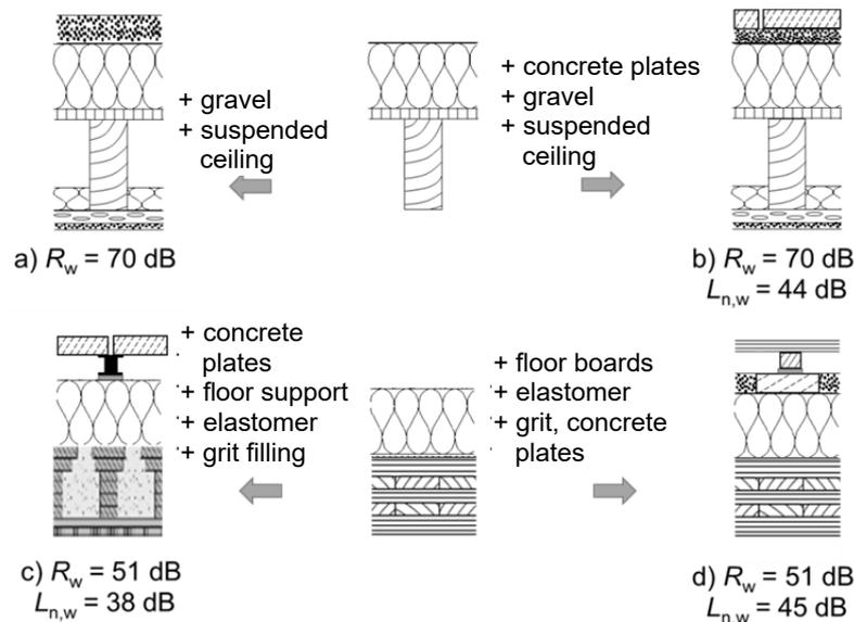
**Figure 1** Flat roofs made of raftered or solid wood elements with different roofing materials.
