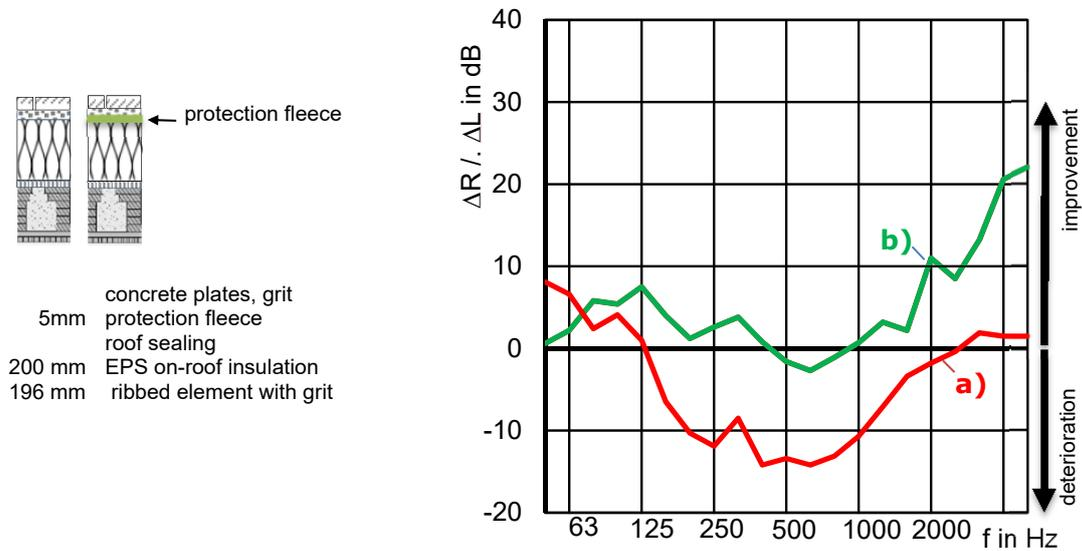
**Figure 5** Improvement of airborne and impact sound insulation by means of a protection fleece from the direct comparison measurement with and without a protection fleece
