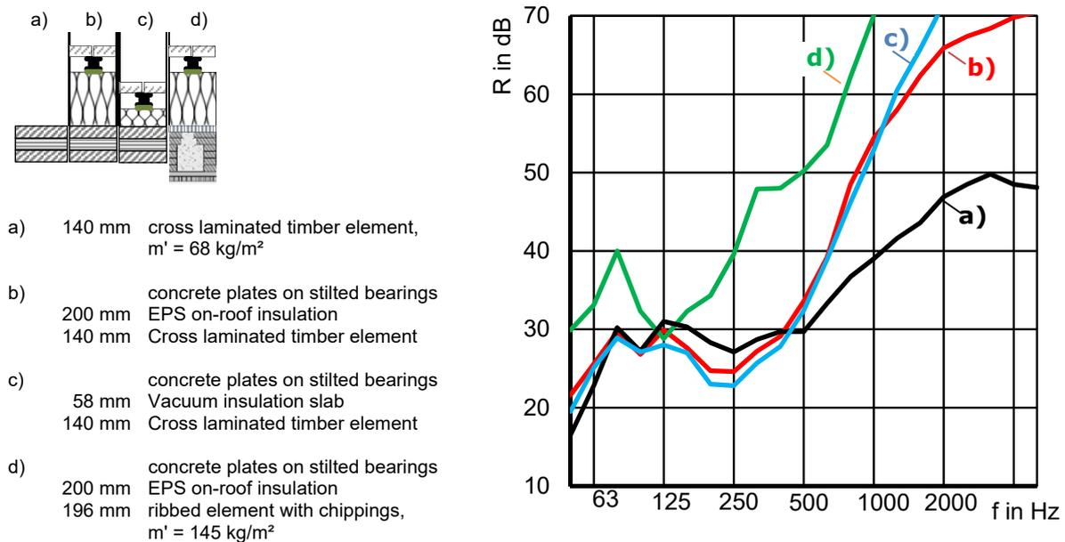
**Figure 3** Influence of on-roof insulation on the sound insulation of flat-roof constructions. The construction above the insulation board (here: 40 mm concrete slabs, support bearings, construction bearings, roof sealing) is not decisive for the airborne sound transmission due to the joints between the concrete slabs.
