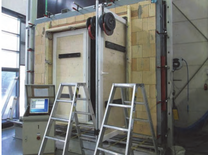
Figure 3 Example of a building element test, here a test set-up for measuring the deformation by simulating the vertical payload
