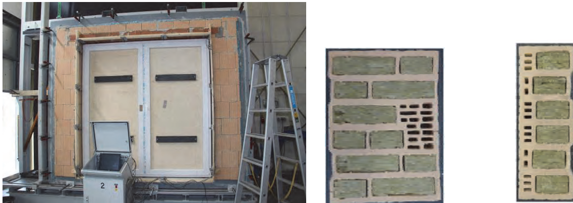
Figure 9 Sample wall design with window element as well as the reveal bricks used
