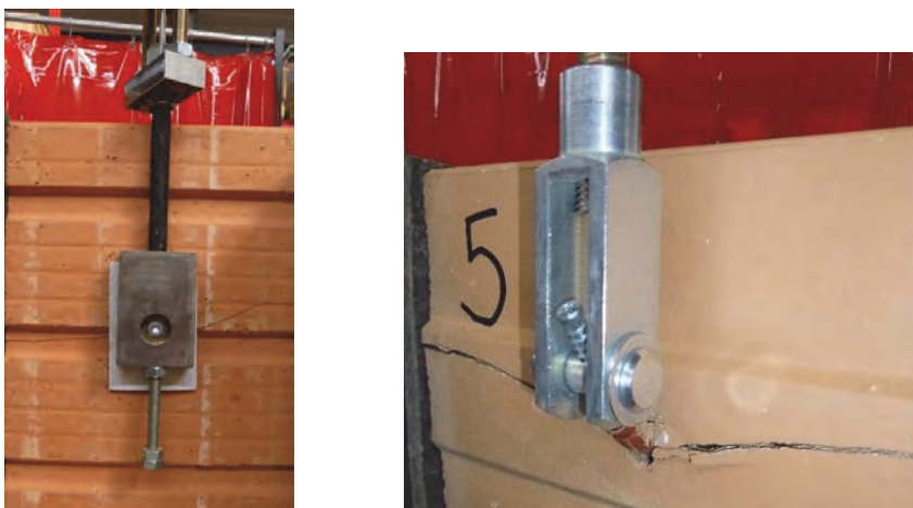
Figure 2 Test for determining the load-bearing capacity of the fastening Left: Purely transverse tension Right: Tensile test with bending of the fixing material
