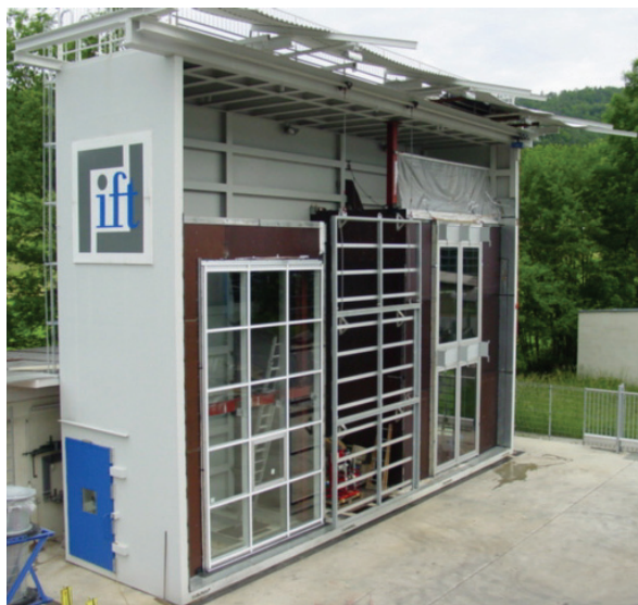
Fig. 3 Facade test rig of the ift Rosenheim
