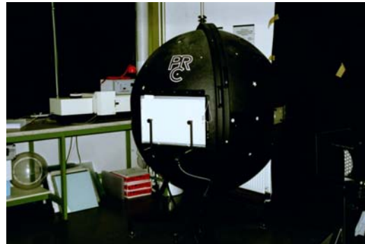
Picture of the integrating sphere at ift Rosenheim
