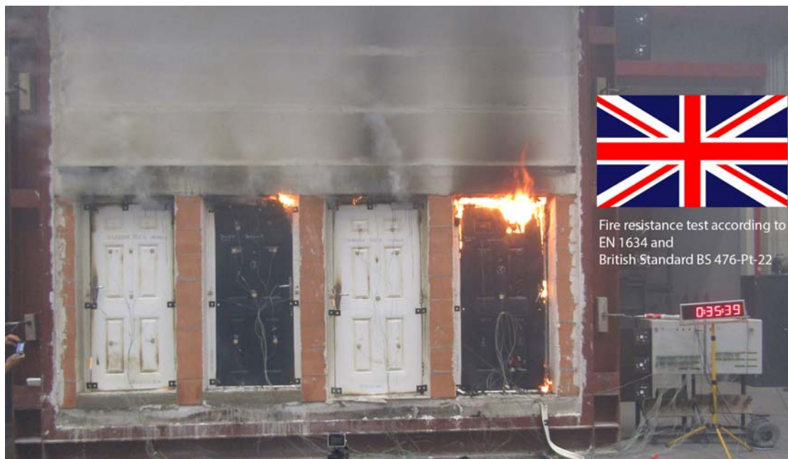
Fig 4 "On Her Majesty's behalf" 100 doors are tested for fire resistance in accordance with EN 1634 and British Standard BS 476-Pt-22 at the Rosenheim Fire Protection Centre.
