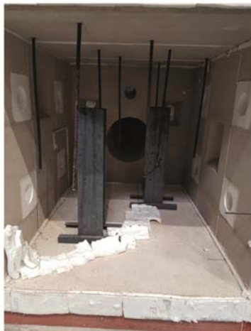
Small Scale Furnace Vertical (1,5 m × 1,5 m), Horizontal (1,5 m × 2 m) Testing according to ETK-, UL-, HC- and RWS-curve, unloaded
