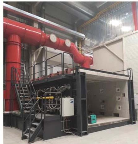
Floor Furnace Testing of horizontal (5 m × 4 m) and vertical (4 m × 2,5 m) loaded/unloaded components according to ETK-, UL-, HC- und RWS-curve. The load is applied with 16 cylinders á 5 tons, 10 cylinders á 10 or 20 tons (not more than 60 tons per bracket).
