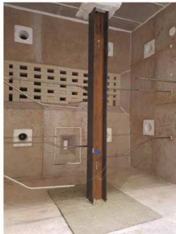
Column Furnace 3 m × 3 m × 3 m, Testing according to ETK-, UL-, HC- und RWS-curve, oaded/unloaded up to 500 tons
