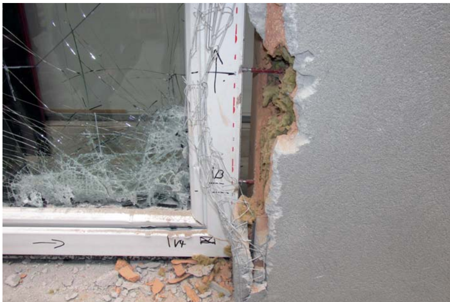
Fig. 2 Example attack on reveal with RC2 tool
