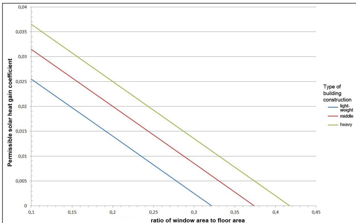
Fig. 1 Permissible solar heat gain coefficients for non-residential buildings
