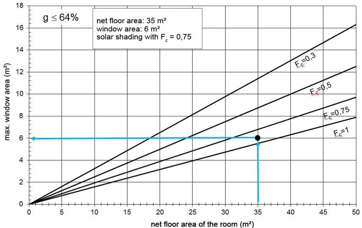
**Fig. 2** Verification of thermal insulation in summer – residential building with thermal insulation glazing
